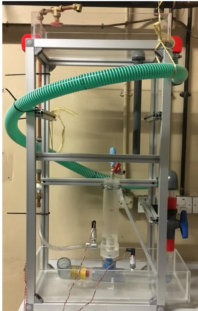
Figure 6: The ram pump after increasing the length
