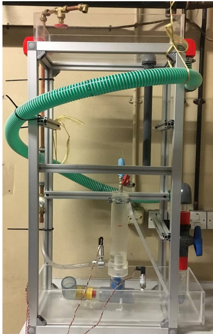
Figure 6: The ram pump after increasing the length
