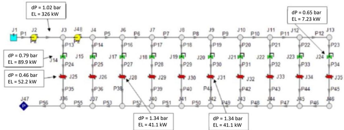
Figure 3 – Case D2 layout and results for the distribution system
