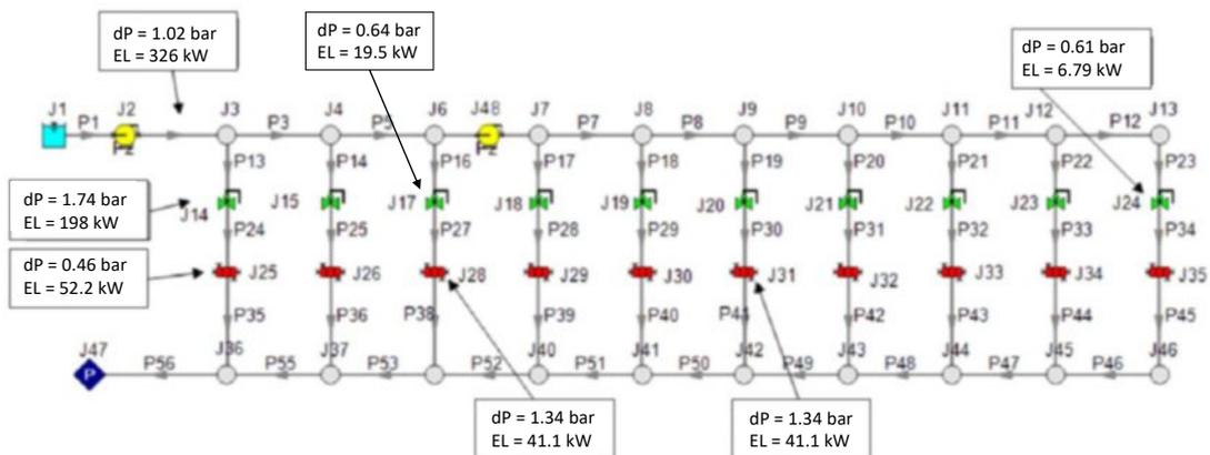
Figure 6 – Case D3 layout and results for the distribution system
