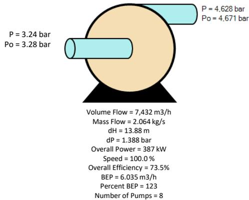
Figure 5 – Case D2 results for auxiliary pumping system
