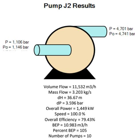
Figure 2 – Case D1 results for the pumping system
