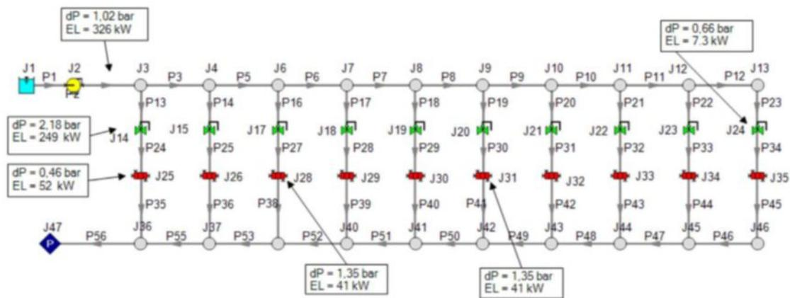
Figure 1 – Case D1 layout and results for the distribution system
