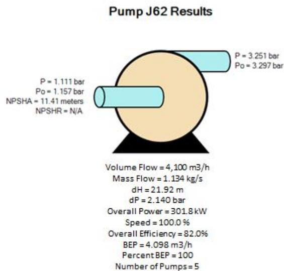
Figure 10 – Case D4 results for first pumping system
