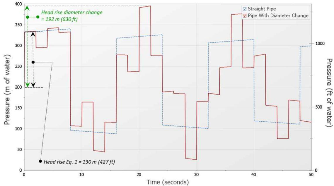
Figure 12: Example 5 - Simulation results for Figs. 7 and 10 at the valve for straight pipe and pipe with diameter change systems.
