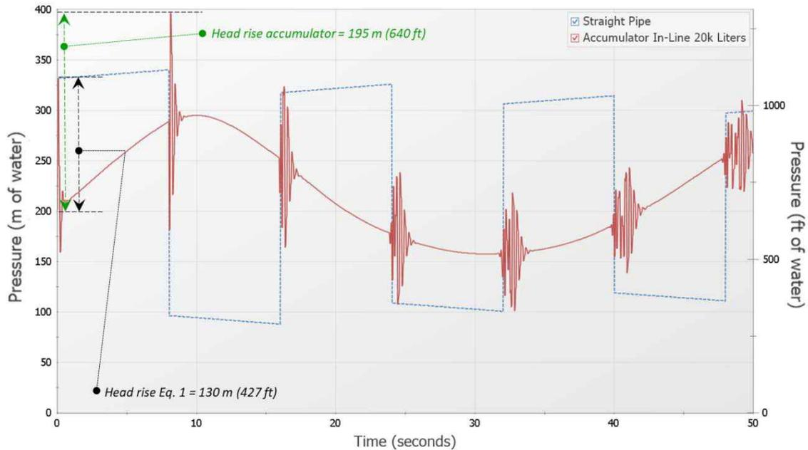
Figure 16: Example 7 - Simulation results for Figs. 7 and 14 at the valve for straight pipe and gas accumulator systems
