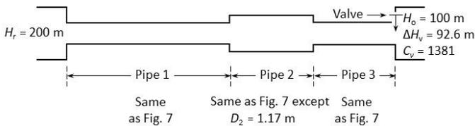
**Figure 10: Example 5 - Piping system with diameter change**
