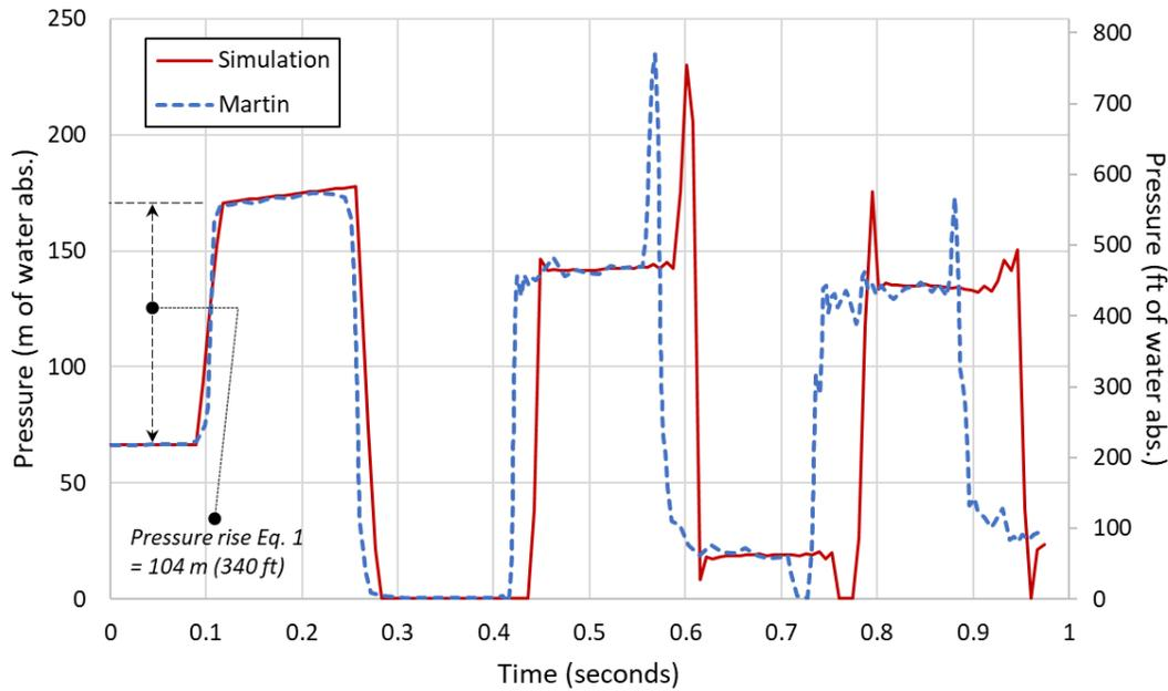
**Figure 1: Example 2 - Experimental and numerical predictions of pressures during transient cavitation, compared to the maximum predicted Joukowsky pressure (Eq. 1)**
