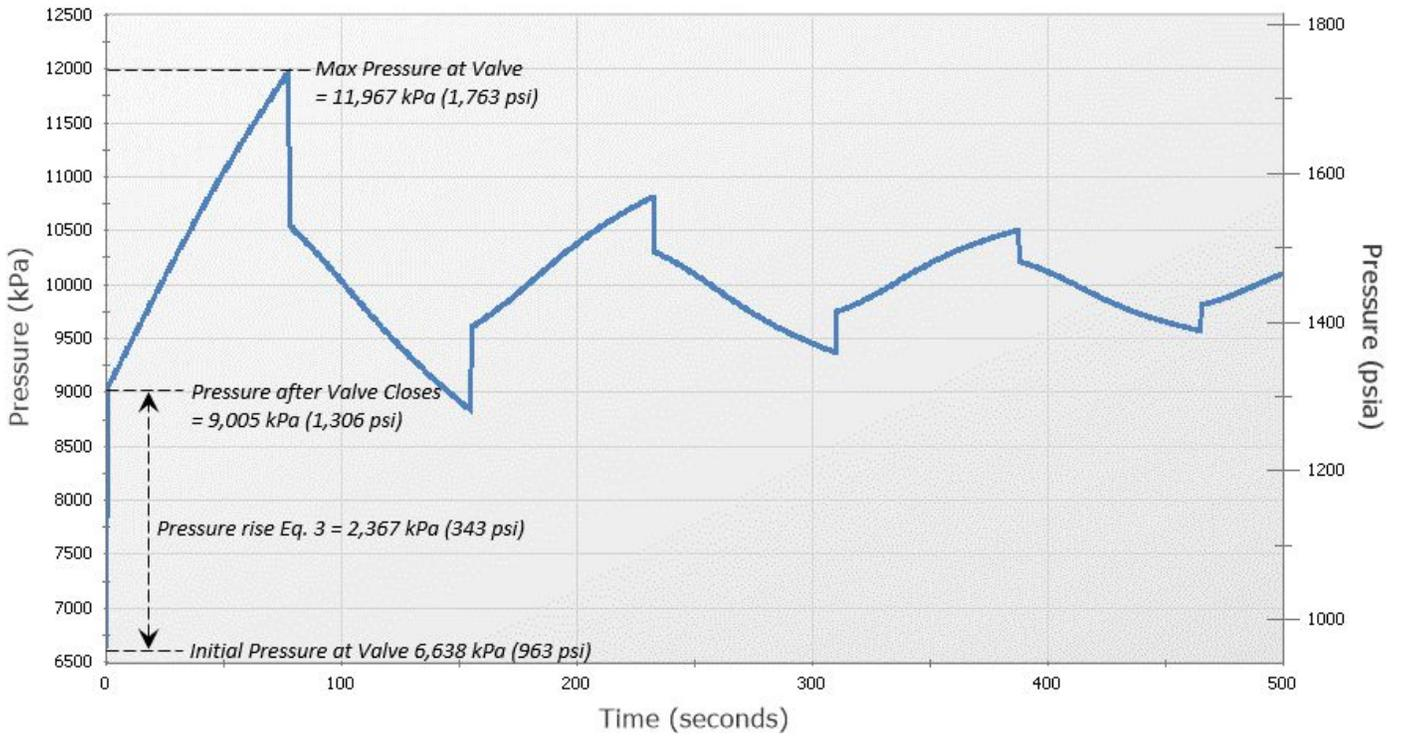
Figure 4: Example 3 - Predicted pressure transient at the valve for the system shown in Fig. 3 for 500 s
