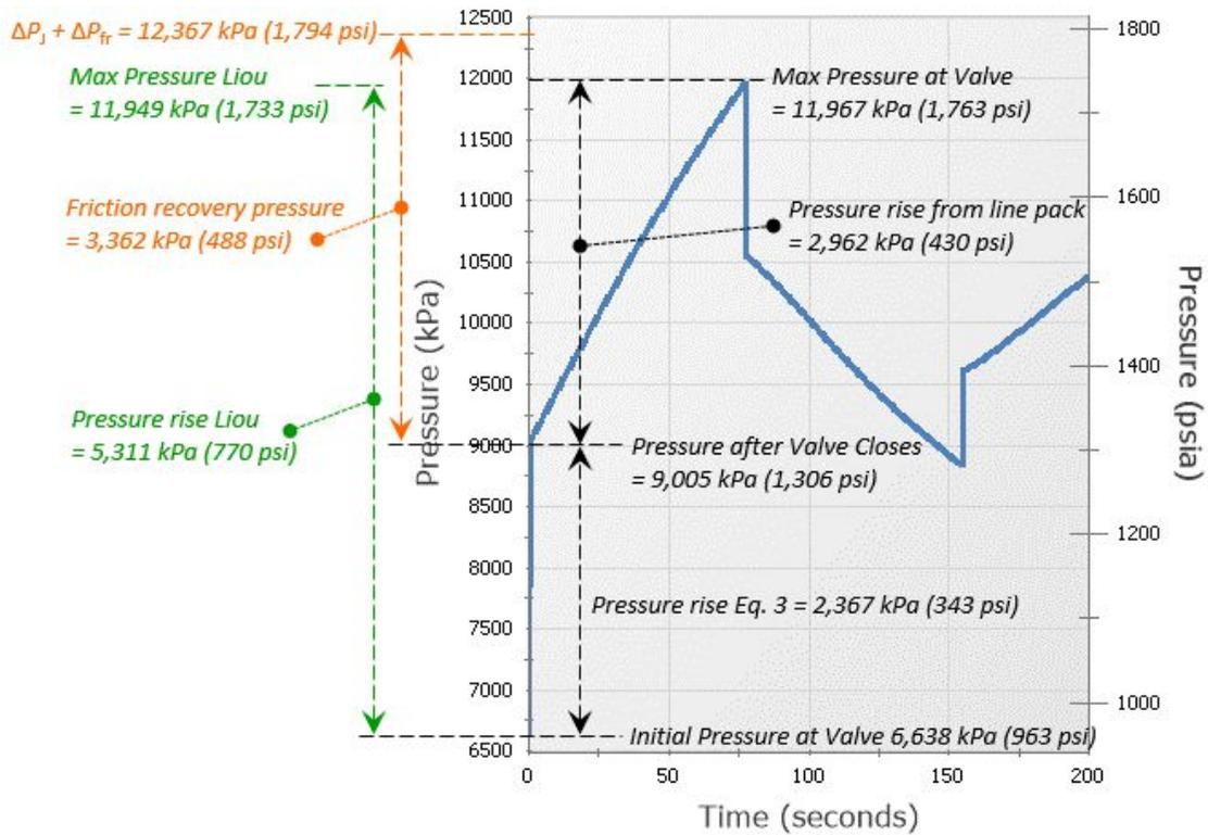
Figure 5: Example 3 – Predicted pressure transient at the valve from the system shown in Fig. 3 for 200 s with additional details on the various pressure rise estimation methods
