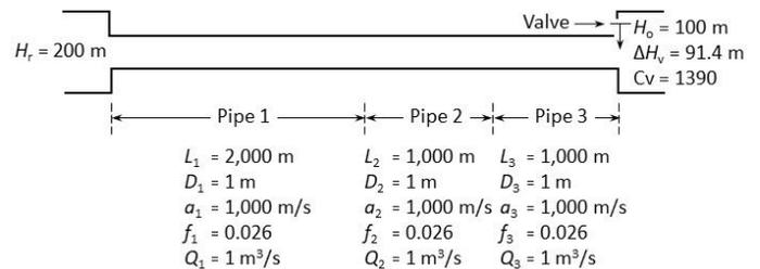
Figure 7: Example 4 – Straight piping system
