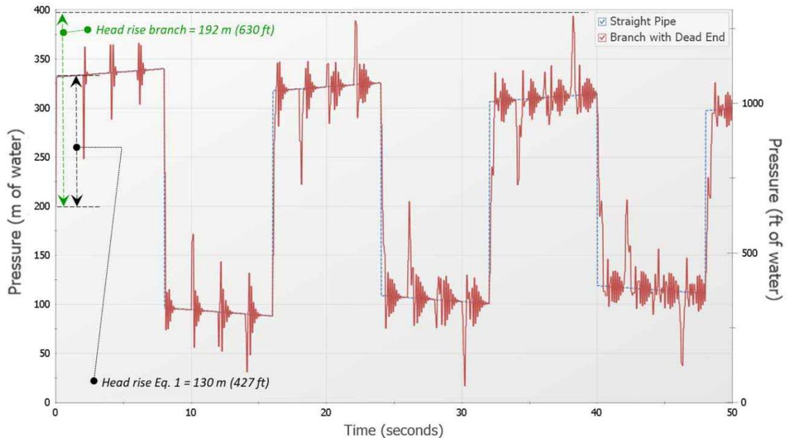
Figure 13: Example 6 - Simulation results for Figs. 7 and 11 at the valve for straight pipe and branch with dead end systems.
