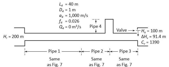
**Figure 11: Example 6 - Piping system with a branch and dead end**
