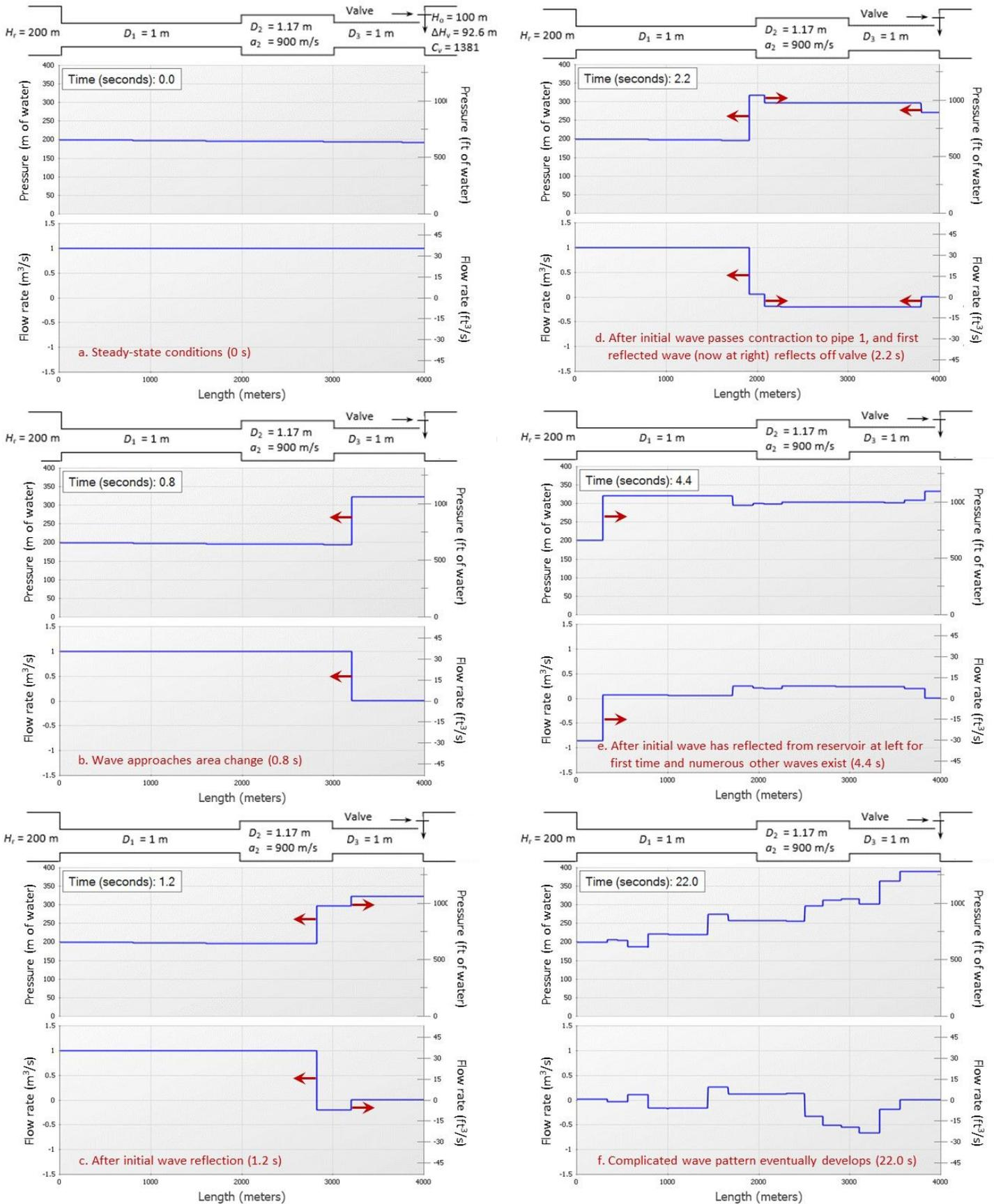
Figure 15: Simulation results at various simulation times for the Fig. 10 system (with wave speed changed in Pipe 2 to 900 m/s) showing pressure and flow rate profiles and how wave patterns become more complicated over time
