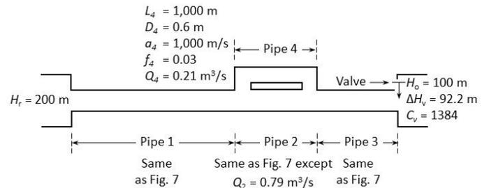
Figure 8: Example 4 - Networked piping system
