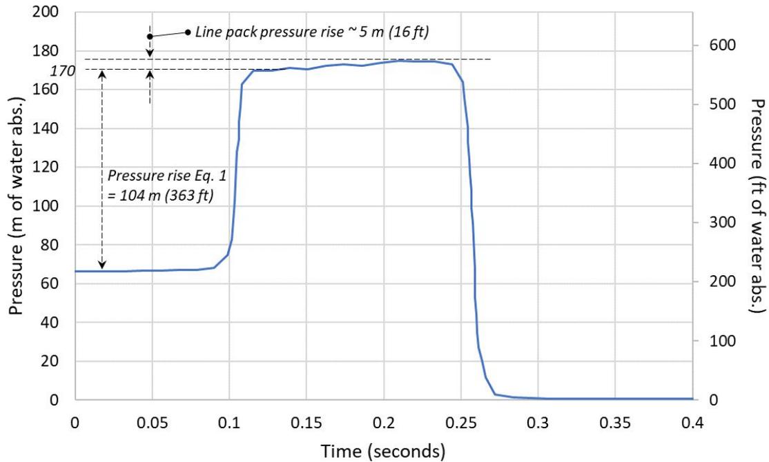
Figure 6: Example 2 - Evidence of line pack effect in experimental results (Martin [12])
