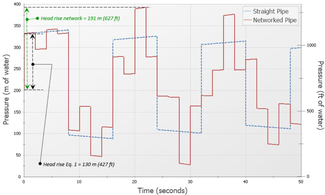
**Figure 9: Example 4 - Simulation results using [11] for Figs. 7 and 8 at the valve for straight and networked systems (adapted from Karney and McInnis [16])**
