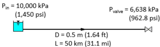
Figure 3: Example 3 – Horizontal pipe system description
