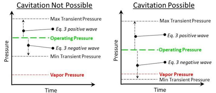
**Figure 2: Diagram to help determine the possibility of transient cavitation**
