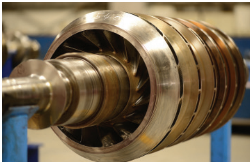
FIGURE 3. Centrifugal compressors can generate different steady-state flowrates with a single motor speed
