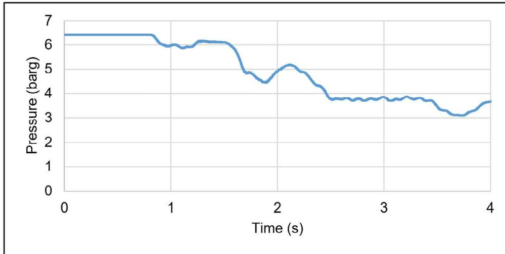
**Figure 9: Top of riser pressure with surge vessels**
