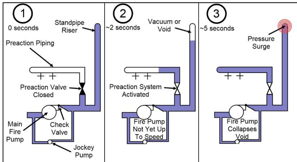
**Figure 1: Steps of void formation and collapse during activation of preaction system**
