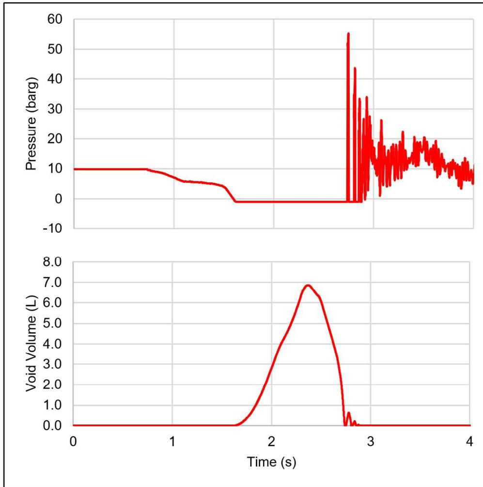
**Figure 6: Cooling yard hydrant pressure and void volume with no mitigation**
