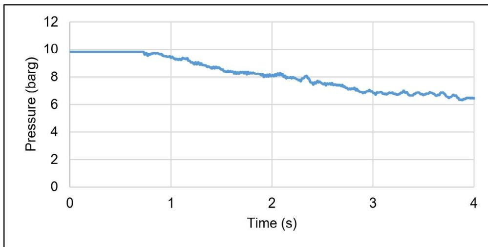
**Figure 10: Cooling yard hydrant pressure with surge vessels**
