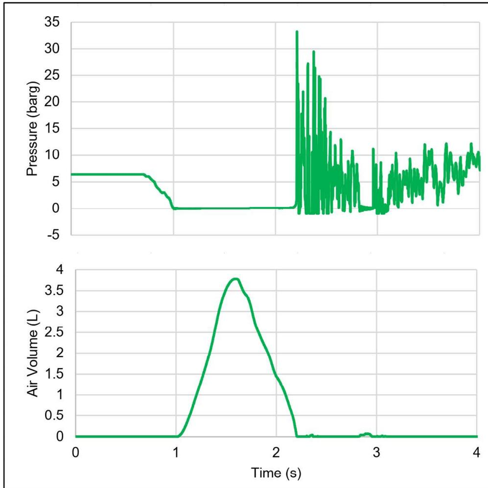
**Figure 7: Top of riser pressure and air volume with vacuum breaker valve**
