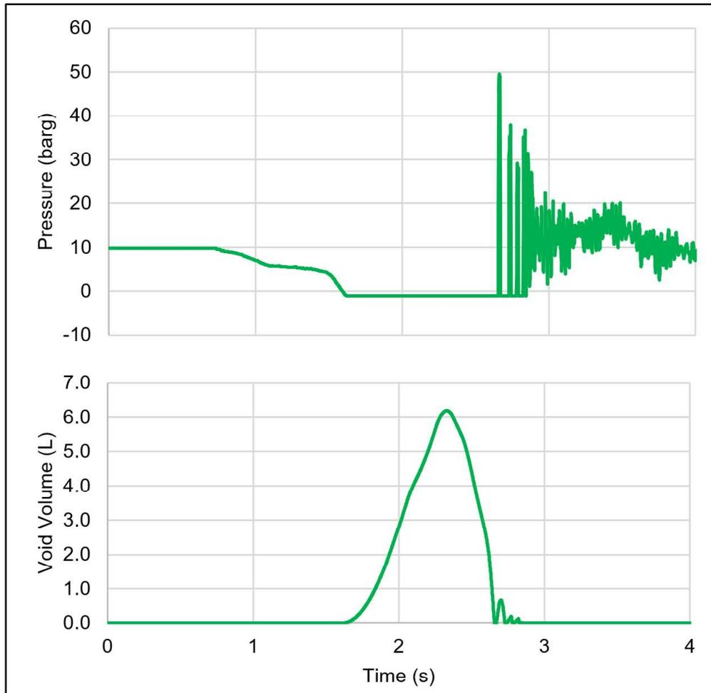
**Figure 8: Cooling yard hydrant pressure and void volume with vacuum breaker valve**
