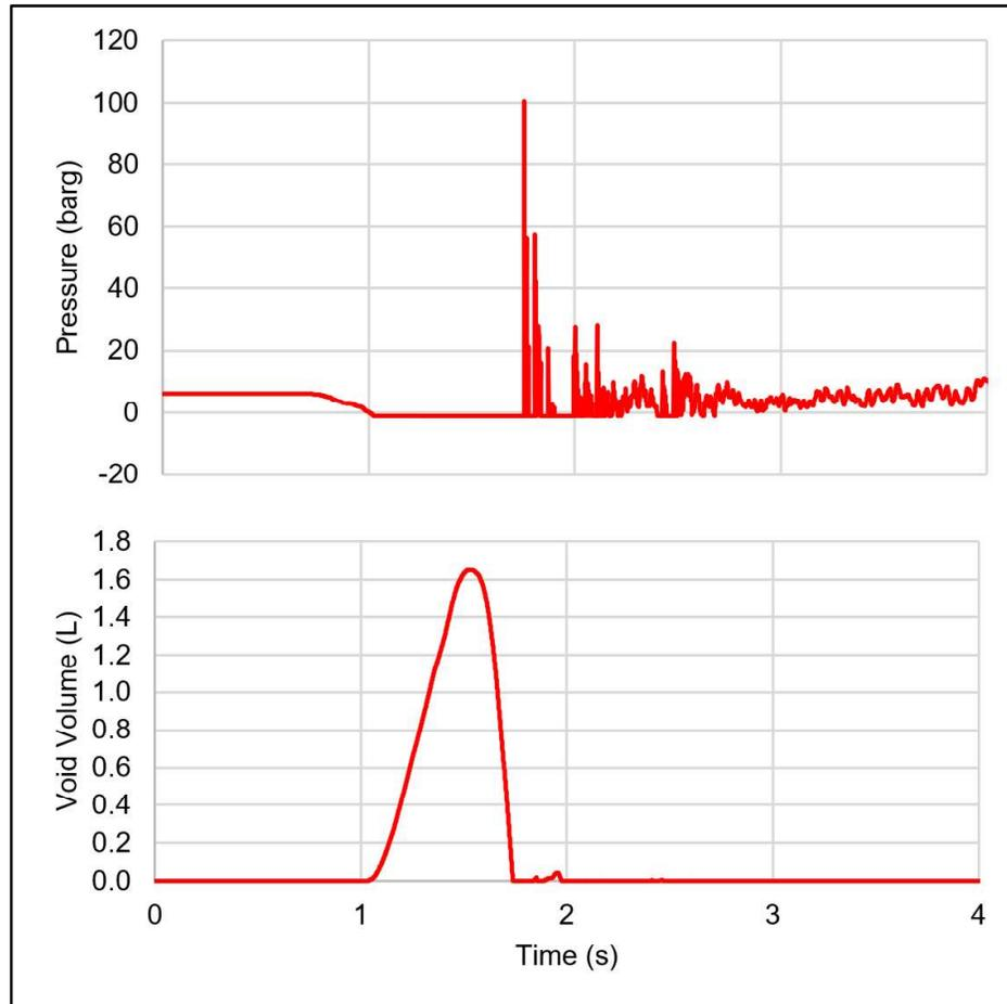
**Figure 5: Top of riser pressure and void volume with no mitigation**
