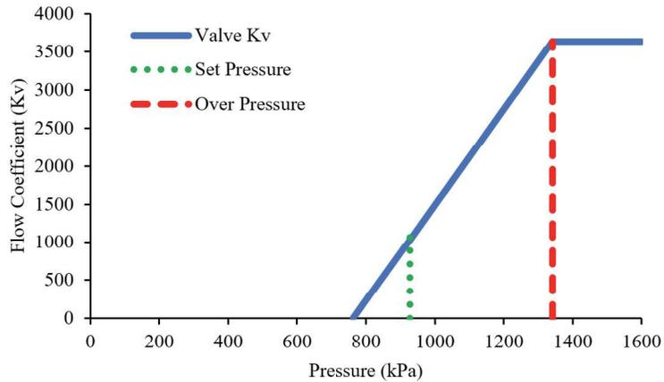
**Figure 1: SRV flow coefficient vs. pressure**
