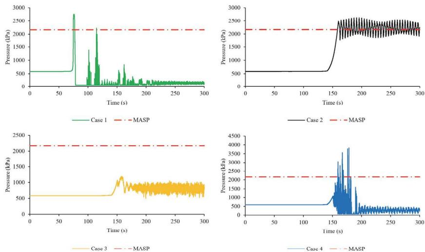
**Figure 8: Pressure at inlet of 750 mm gate valve**
