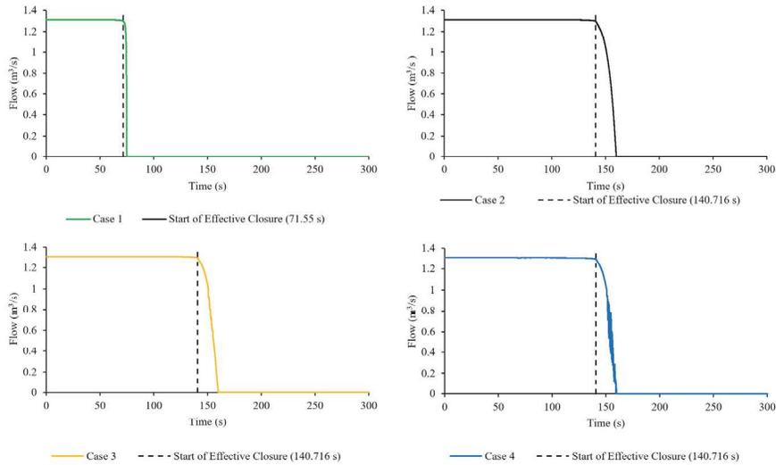
**Figure 7: Flow at inlet of 750 mm gate valve**
