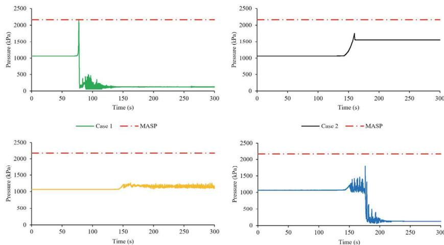
**Figure 10: Discharge pressure at one pump**
