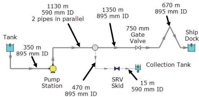
Figure 5: Simplified model view of flow path and relief line
