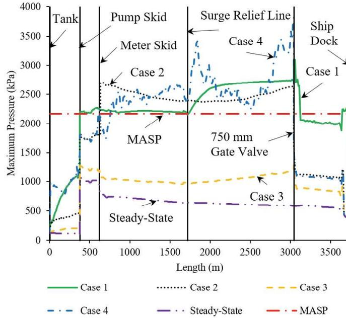
**Figure 6: Steady-state pressure, maximum pressure envelopes, and maximum allowable surge pressure (MASP)**
