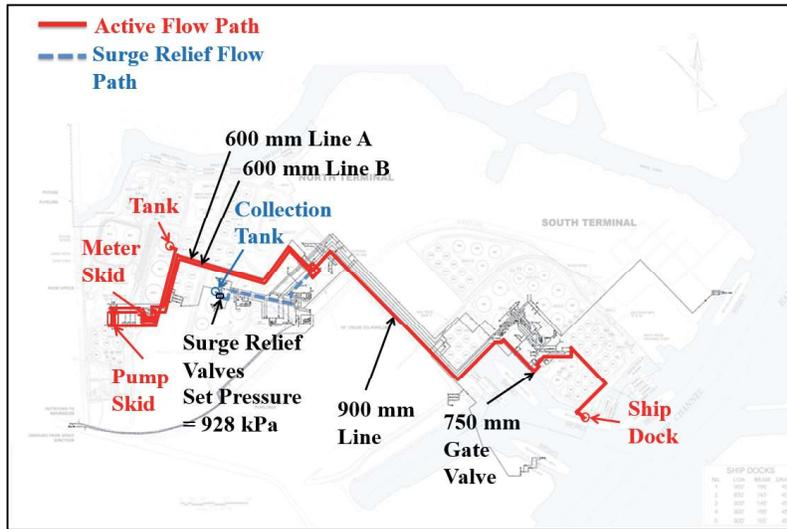
Figure 4: Active flow path and surge relief path for cases 1, 2, 3, and 4
