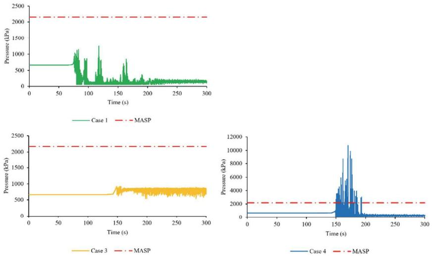
**Figure 12: Pressure at inlet of one relief valve**
