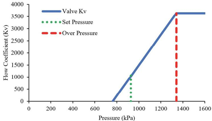
**Figure 1: SRV flow coefficient vs. pressure**
