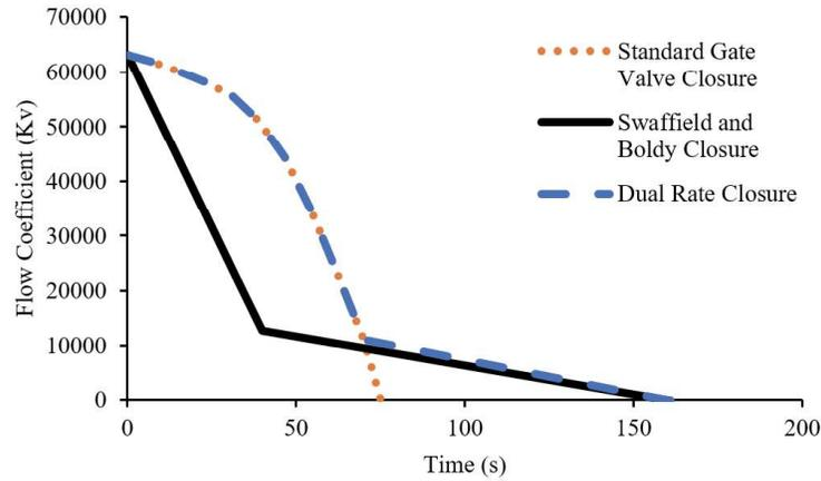
Figure 2: 750 mm gate valve closure profiles
