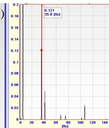
Fig 10. Natural Frequencies and Mode Shapes – based on FFT of 4 seconds following Fig 7 Impact
